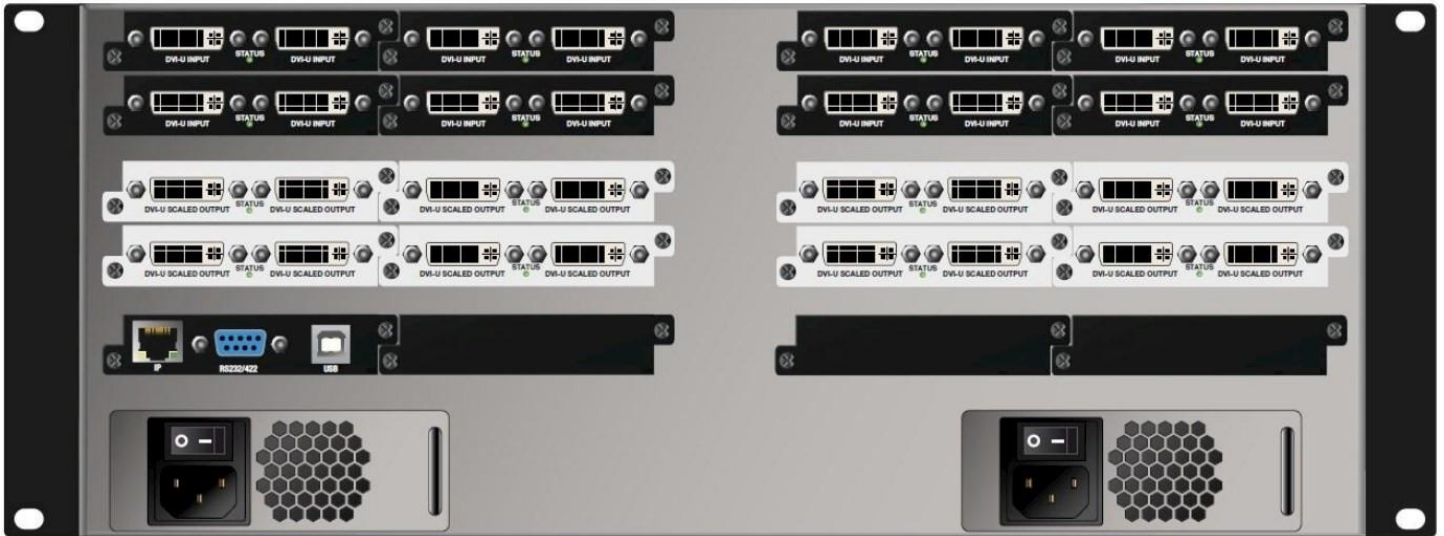
8 Universal DVI Inputs, 8 3G-SDI/HD-SDI/SD-SDI Inputs, 16 Standard DVI-I Outputs
